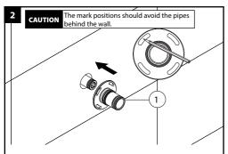
Place MOUNTING ADAPTER (1) onto the faucet as shown. Using the MOUNTING ADAPTER (1) as a template, mark the positions of the screw holes.
