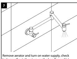
Remove aerator and turn on water supply, check leakages. If not, then turn on the handles and let water run for at least one minutes, this will clear any debris left in the line, reinstall the aerator.
