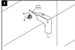
Drill 3/32" holes where marked. If using the anchors, drill 1/4" holes.
